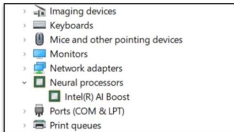
2. **If an NPU driver is installed, you need to uninstall it.**
