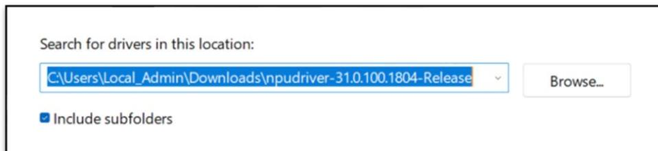
8. After setting the correct location tick the **Include Subfolders** checkbox and click *Next*. The driver will now install.
