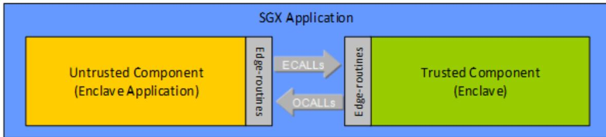
The first step in designing an Intel SGX enabled application is to identify the assets it needs to protect, the data structures where the assets are contained, and the set of code that operates on those data structures and then place them into a separate trusted library. Since the ISV knows the application best, the ISV should conduct a security analysis of the application and properly partition it making the decision about what code and data is placed in the enclave.
